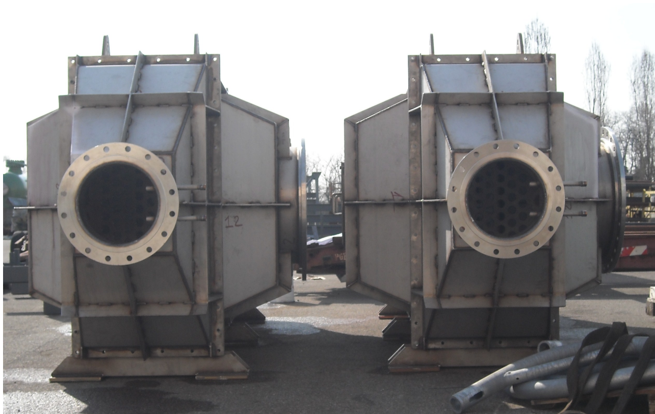
Air-air exchanger fully made in stainless steel AISI 316L (Kazakhstan Caspian sea)
